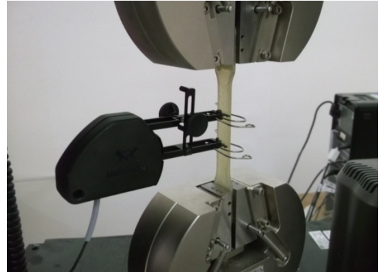
Fig. 2. Specimen between the jaws of machine with the extensometer.
